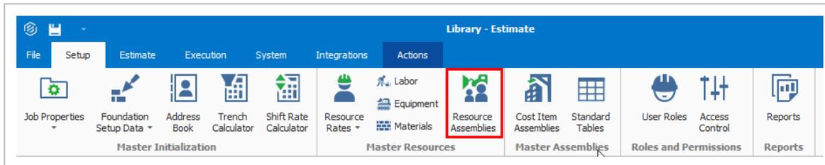
The most common use for an assembly is to group labor resources into crews (e.g., Pipe Crew, Concrete Crew); however, any resource (equipment, materials, etc.) may be grouped into an assembly. Utilizing assemblies allows you to estimate faster, since you can add and manage an entire group of resources at once.
